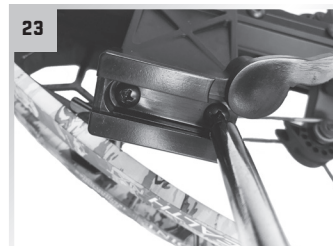
Install the quick disconnect (female) attachment.
