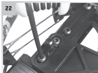
Insert and tighten two 1/4-20 x 3/4-inch button-head cap screws.
